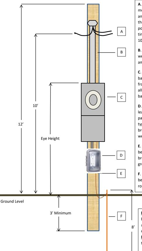
A. <u>Weather Head</u> The weather head must be within 2' of the top of pole and have at least 18" wire extending through the weather head for the power company to connect to. At no time shall the drop loop be less than 10' of the ground.
